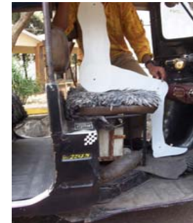
5 th % (males) have problem reaching floorboard Brake lever in awkward position
