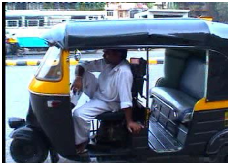
The rickshaw driver has to change posture while the rickshaw is idle because of bad seat design.
