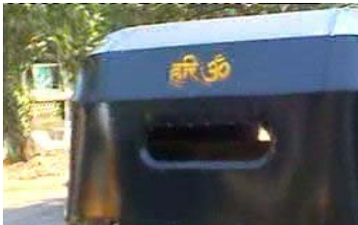
Negligible rear window area, which doesn't give any view to the driver
