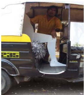
Legroom adequate for two passenger in erect position Inadequate for three passengers and/or relaxed postures
