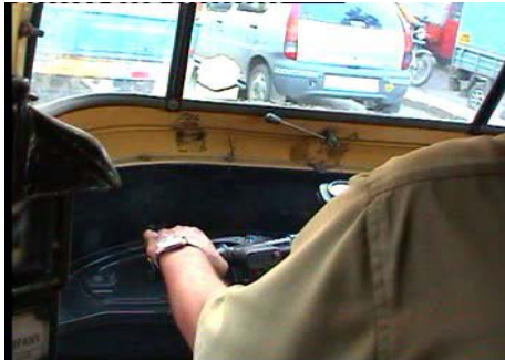
Brake lever too hard which leads to wrist ache
