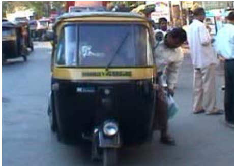
Passenger has to bend down to get in or out
