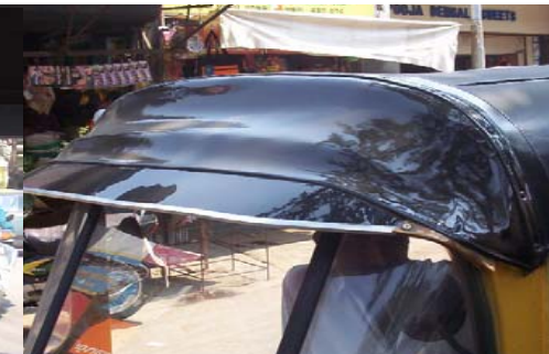
Sunshade reduces the visibility as well as increases air friction
