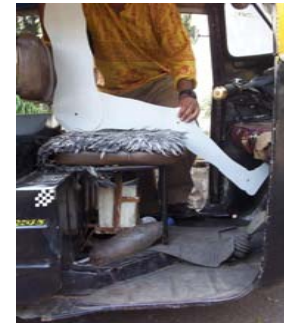
Backrest too far for 5 th % (male) due to improper popliteal width of the seat
