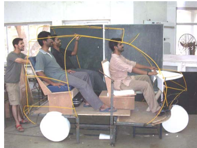
Full scale mock up rig for study purpose and finer refinement
