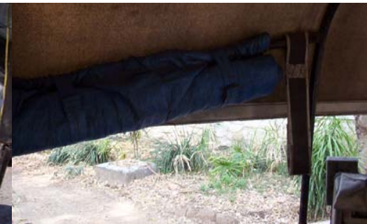
Canopy stretched too much downward, obstructs vision Loose and flexible strap for holding
