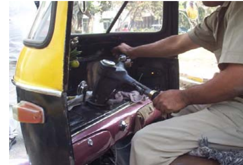
Handle lock broken intentionally to reduce turning diameter Handle hits front panel when turned more Handle hits knees on turning
