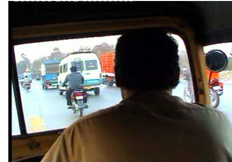
Driver always sits in a very cramped position because of handle bar position, visibility, seat design etc.
