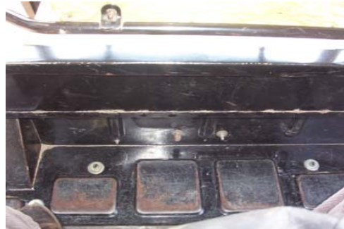
Pressed floor board to give strength, but grooves accumulate dirt.
