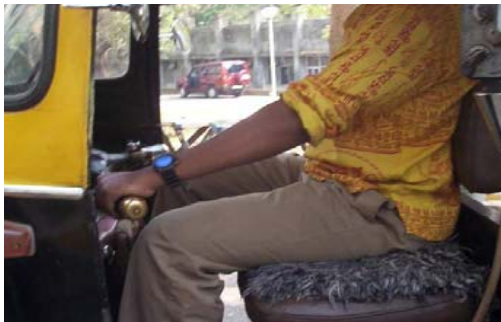
Handlebar is too close to knee Turning difficulty Cramped seating posture due to low handle bar and less legroom
