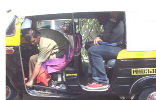
Very tiring posture to start the vehicle if not working within 2/3 pulls
