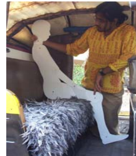
Legroom adequate for two passenger in erect position Inadequate for three passengers and/or relaxed postures
