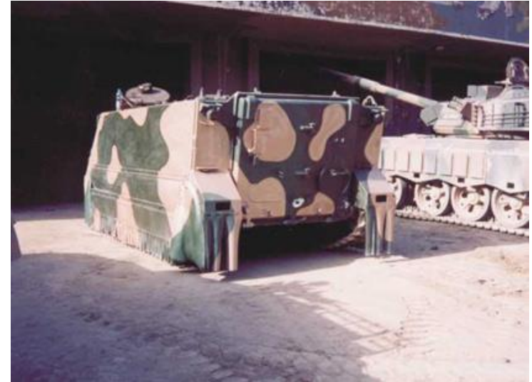
M113 painted with Intermat anti-thermal coatings
