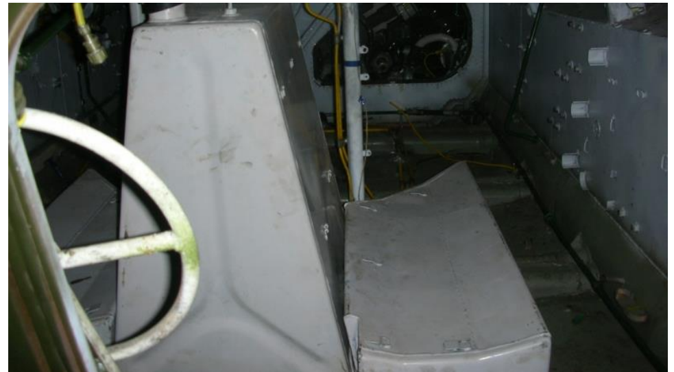
No Harness & Cushioning on the Seats
