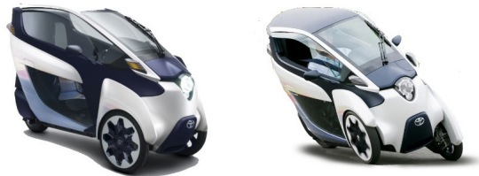
Reverse tilting trike tandem seating 2350/850/1445/1700
