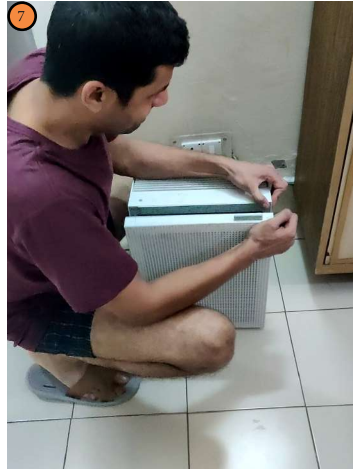
Img. 7 No provision for Hatch opening so the user has to forcefully insert finger nails between the gaps, No AQI info, No Handle
