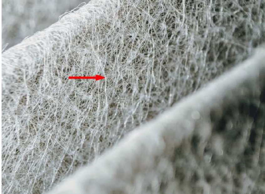
fig. 9 HEPA filters fiberglass fibers under a microscope.
