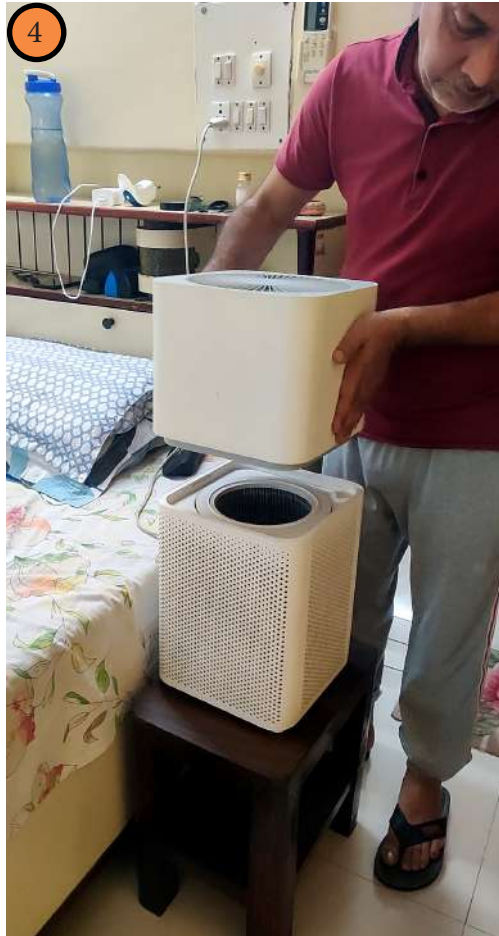
Img. 4 Hatch opening locks on side, Which can be pressed while lifting the object
