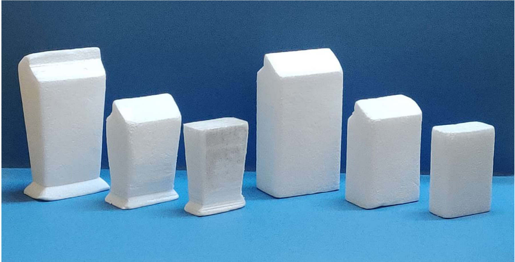
fig. 24 Small Scale Thermocol mockup for Checking Forms
