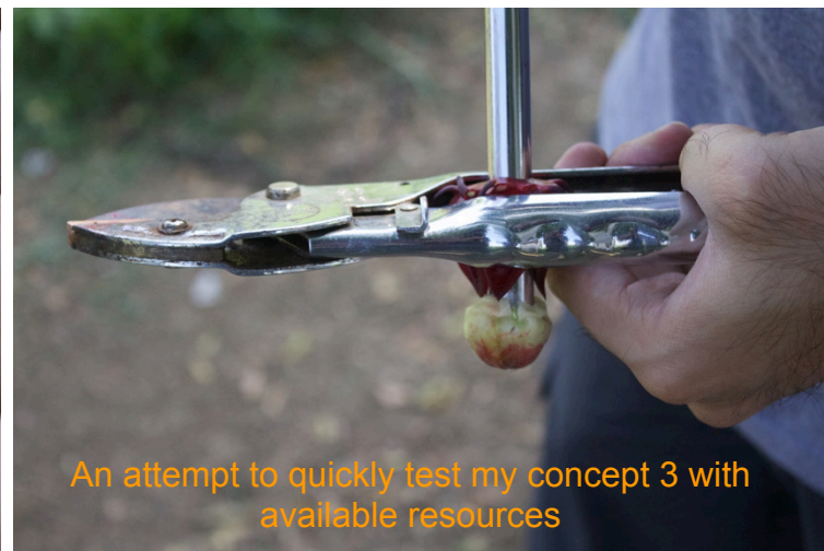
Cutting tool for cutting from stem
