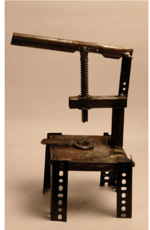
Handle concept with variable height enabled by slotted angles
