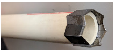
The blade edge mockup which triggered the idea of serrated blade edges
