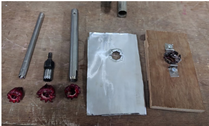
Experiemnt with handmade serrated blade, available blade from repurposed hole-saw and grinded circular pipe
