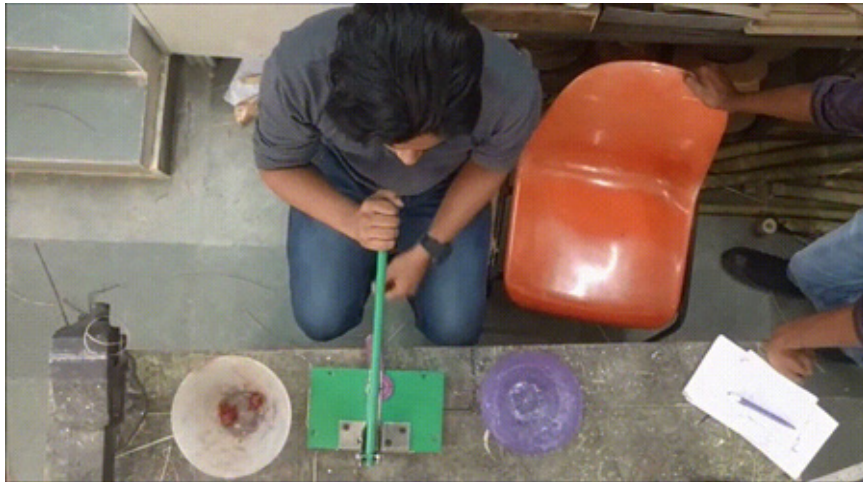
Fresh Ambadi fruit container and calyx container on either sides of machine (slower, requires hand switching)
