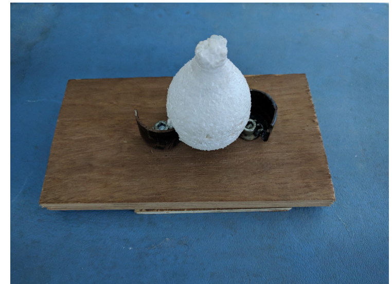
Dummy Ambadi fruit mounted on nails and engaged blades. Once the nails are rotated, the Calyx is expected to fall off leaving the seed pods behind
