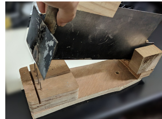
Metal proto with nails as base holder for Ambadi
