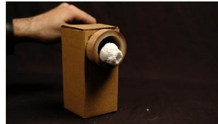
Fruit mounted by hand once onto central nail mounts, then retracted for incision by outer blades until calyxes fall off. (Fruit is not held by hand)
