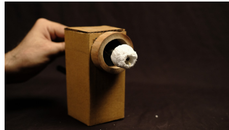
Fruit mounted by hand once onto central nail mounts, then retracted for incision by outer blades until calyxes fall off. (Fruit is not held by hand)
