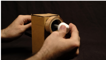
Fruit mounted by hand once onto central nail mounts, then retracted for incision by outer blades until calyxes fall off. (Fruit is not held by hand)
