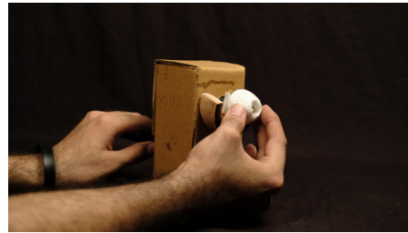
Fruit held with hand, while crank cuts a circular incision on calyxes which eventually fall off
