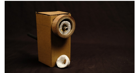
Fruit mounted by hand once onto central nail mounts, then retracted for incision by outer blades until calyxes fall off. (Fruit is not held by hand)
