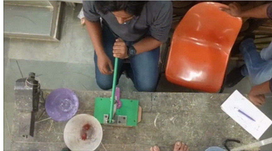
Ambadi fruit and Calyx containers on same side of machine (faster, and does not require hand switching)
