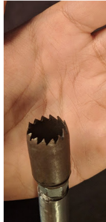
Sharpened 19mm hole saw attached as replaceable blade
