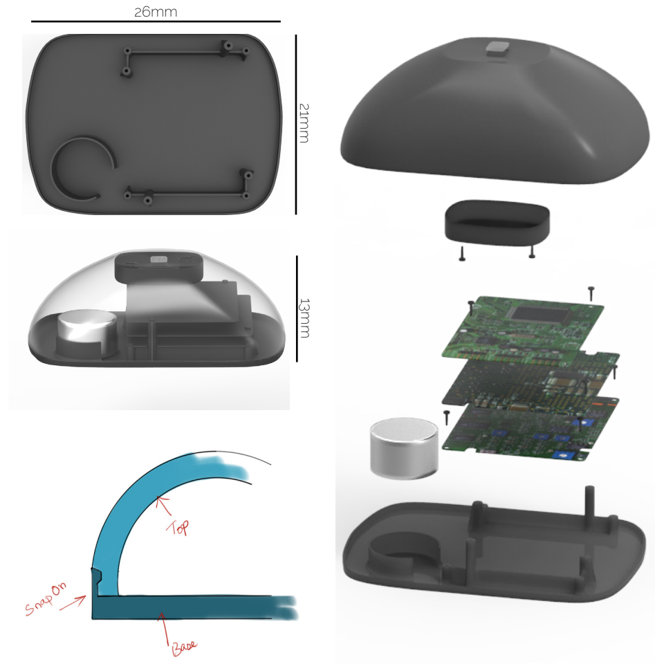
Fig 55 : figure showing the detailing for the packaging of the circuits.
