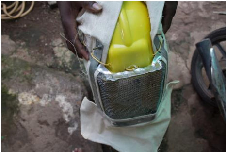
Holes are drilled and tied with the framework and canvas
