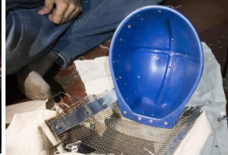
Mesh is bend 90° to the plane of surface of helmet
