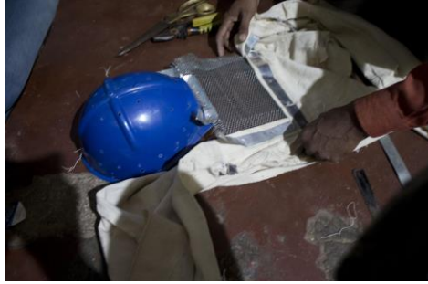
Frame with GI mesh is riveted with the helmet
