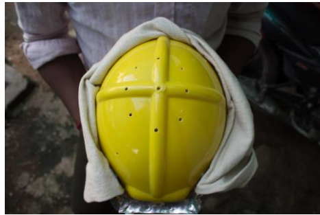
Holes are drilled in the helmet for air ventilation
