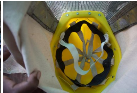
Mesh is bend 90° to the plane of surface of helmet
