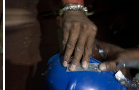
Making the hole in GI sheet from the mark of the hole in the helmet
