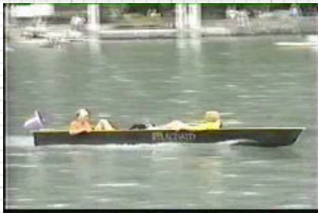
Recumbent face to face position for a double seater craft . helps to dynamically balance the boat
