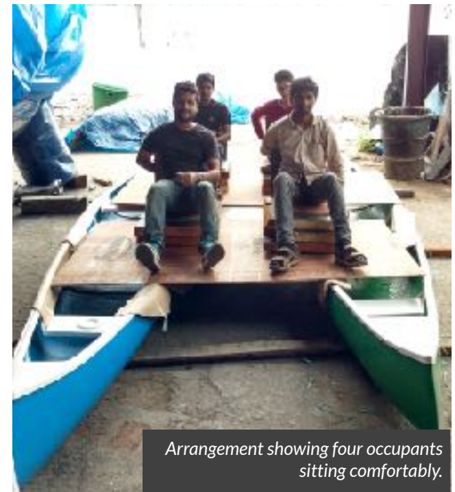
Mock up for finding the dimensions of the deck
