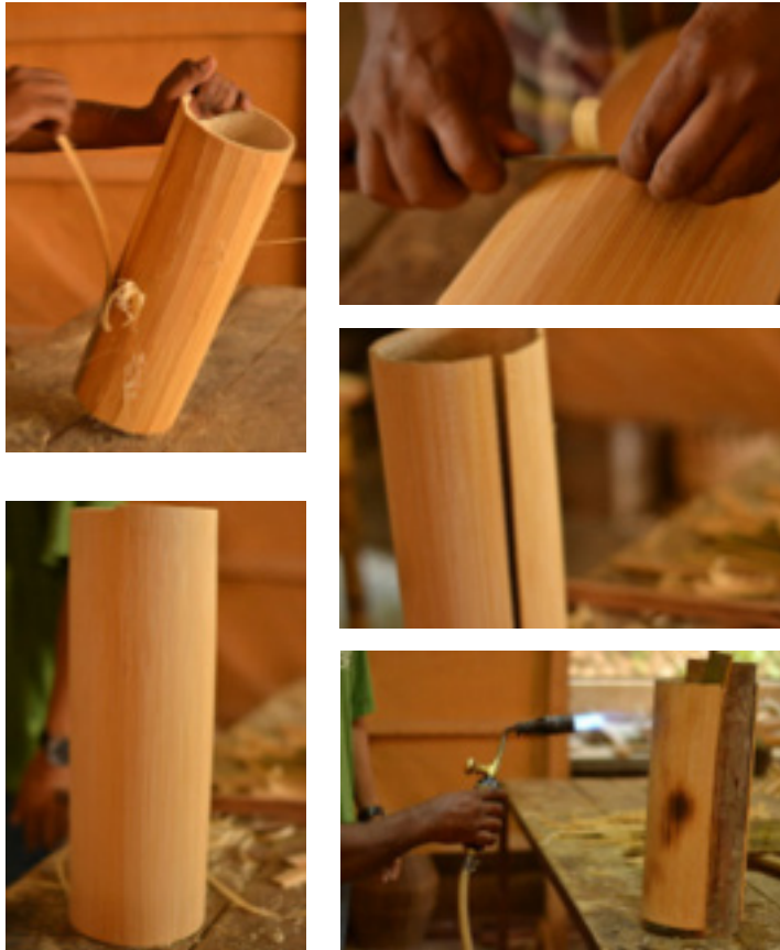
Fig.52: Showing the various stages involved in flattening a bamboo culm
