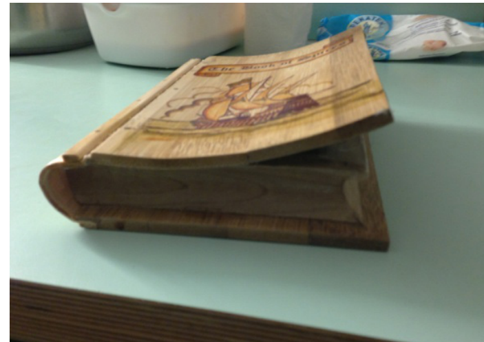
Fig 38: Warping issue at extreme temperatures
