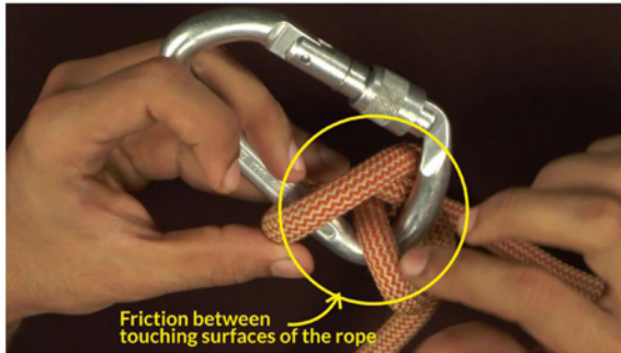
Image: Part of the video explaining the friction between the touching surfaces of the rope
