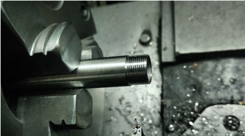
Sensor enclosure with thread. Slit holes are drilled separately
