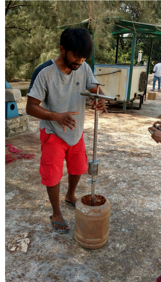
Since the soil selected was too dry it took couple of repeated hammering to achieve desired depth.
