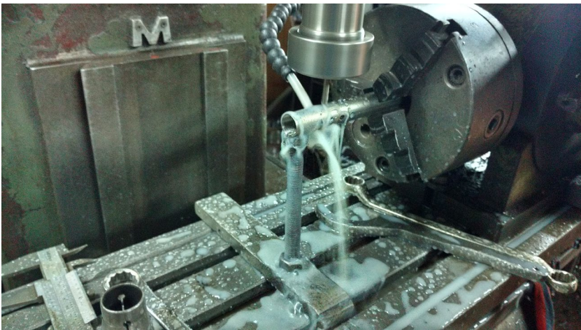
Sensor enclosure with thread. Slit holes are drilled separately
