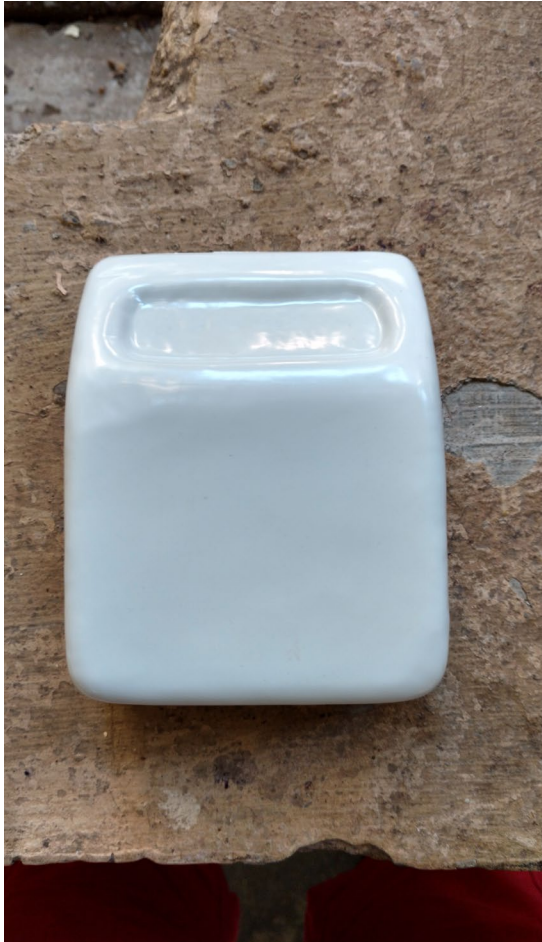
Control unit vacuum formed in styrene
