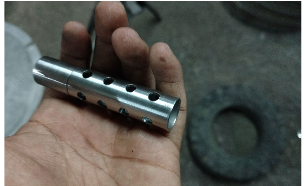
Finished sensor enclosure with slit holes
