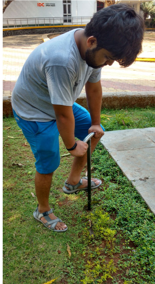
Force is applied over the foot pedal to press down the unit to desired depth
