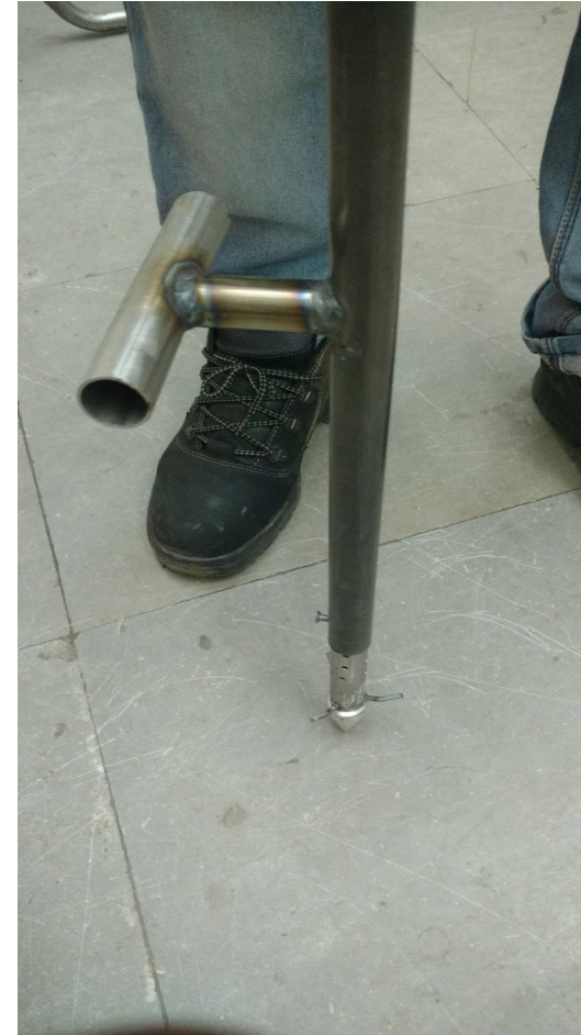
Once the desired depth is achieved, the unit is lifted. The resistance caused results in opening of slotted channel and sensor is exposed
