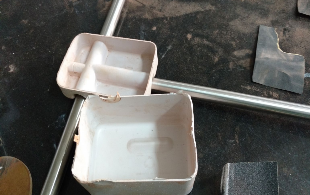
Control box is vacuum formed as two separate halves
