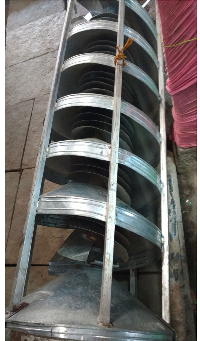
Centrifugal grain separator -Works by centrifugal force that separates grains from impurities
