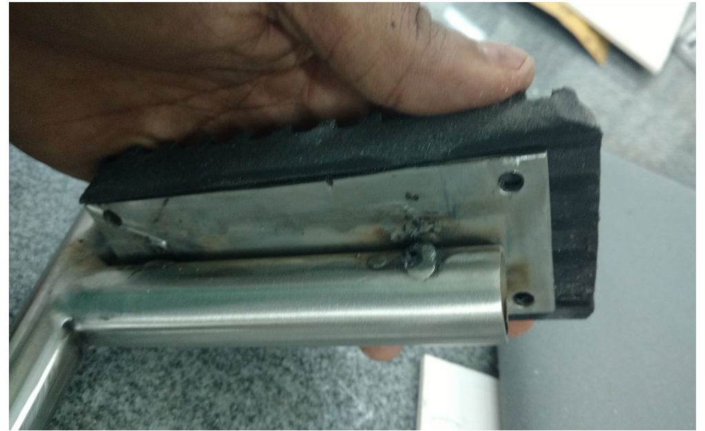
Foot pedal is welded to main pipe and rubber grip is fixed on flat plate
