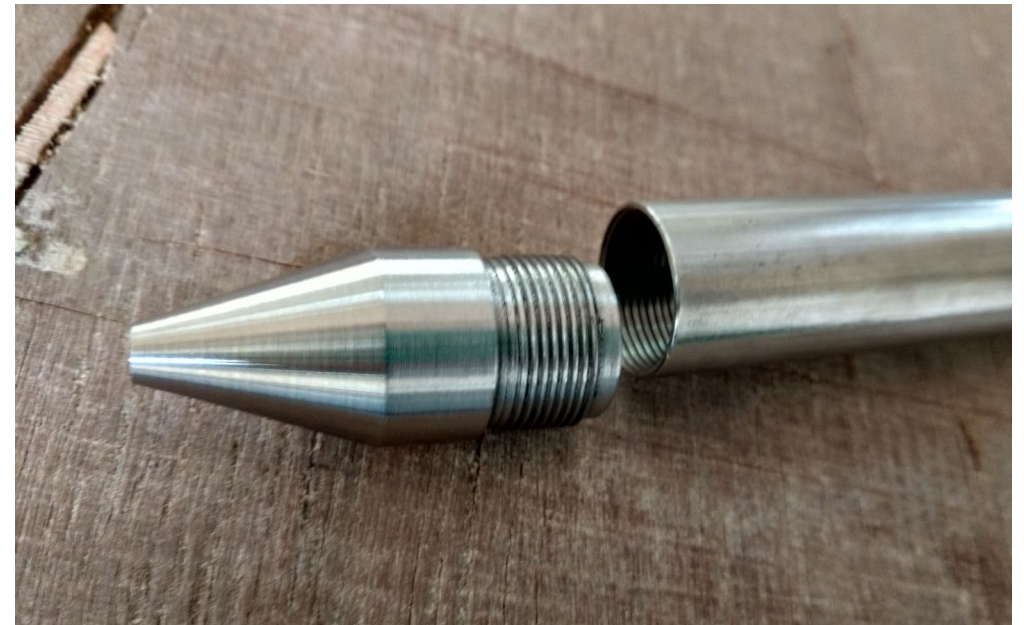
Tapering tip with thread made in lathe
