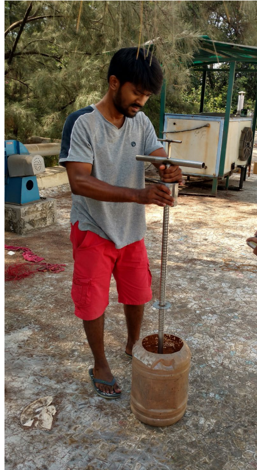
The sliding mass is lifted up and is left to fall freely.
