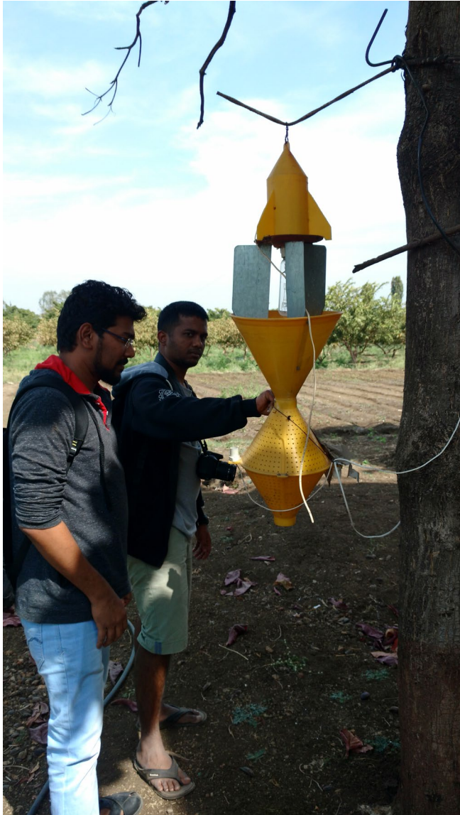
Insect catcher installed in field. -Traps insects with UV light powered by a solar panel
