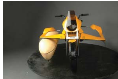
3. The right pontoon is rolled in the side flap
