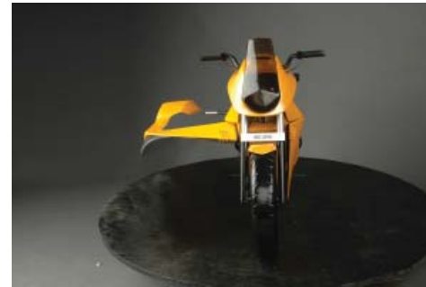
7. The left pontoon is rolled in the left side flap
