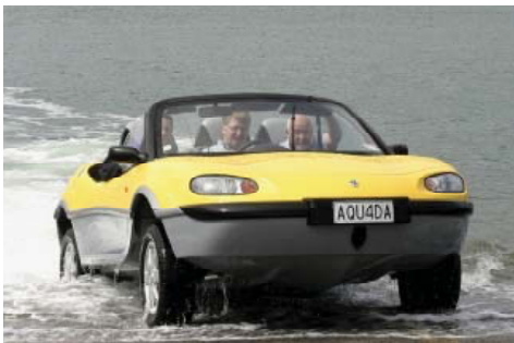
Image 4: Aquada, Year - 2003 looks of a sports car with aerodynamic curved body and hydrodynamically shaped bottom, retractable wheels [6]
