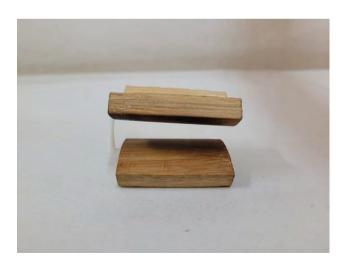
After the preliminary testing I realised that the holes and joinery was too small and lacked the necessary strength. So I made the holes larger by 1mm (to 4mm), which had a significant impact on the strenght.
