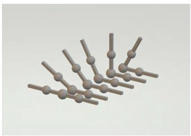
With all of this in place I made some more variations of the bamboo slats, making them with different number of holes, making them in different sizes and drilling lateral holes as another method of joining them.
