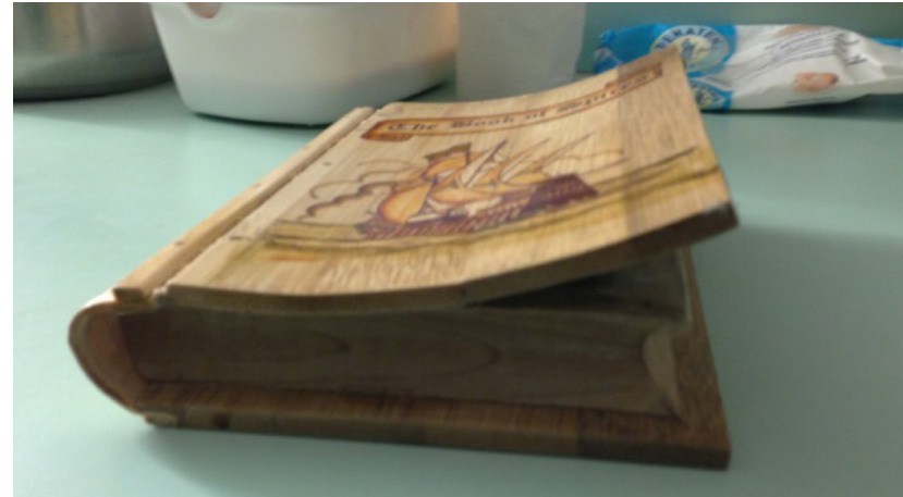
Fig.29: Warping issue seen at extreme temperature; source: Author
