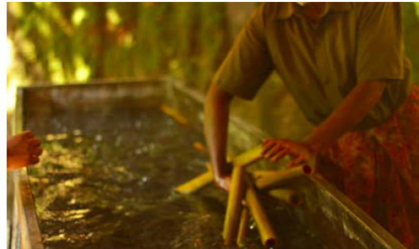
Fig.25: Gas pressure impregnation(top);Hot dipping(bottom); source:Author
