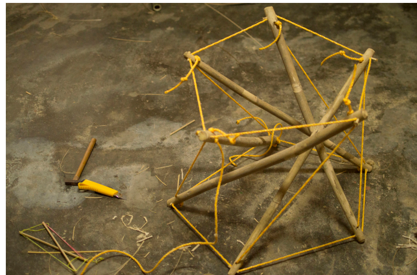
Fig.38: Pentagonal prism before application of tension(top) and after(bottom); source : author
