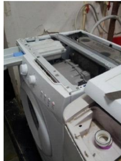
Counterweight supports at front of the drum as well
