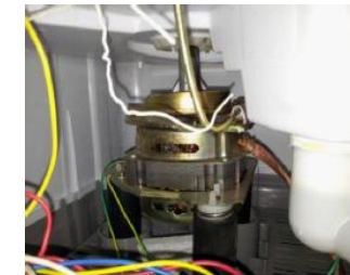
Motor drive for spinning mechanism
