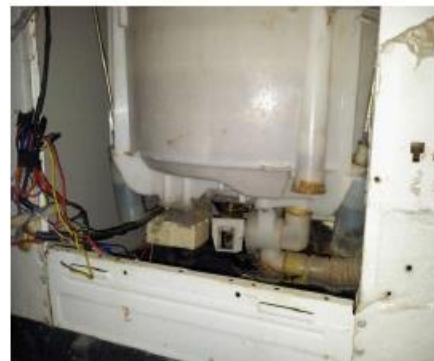
Motor connected to a gearbox for reduction of gear ratio. The gear box is connected to pulsator via a belt pulley mechanism
