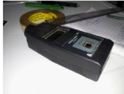
Tacho meter used to decipher the rpm of the machine
