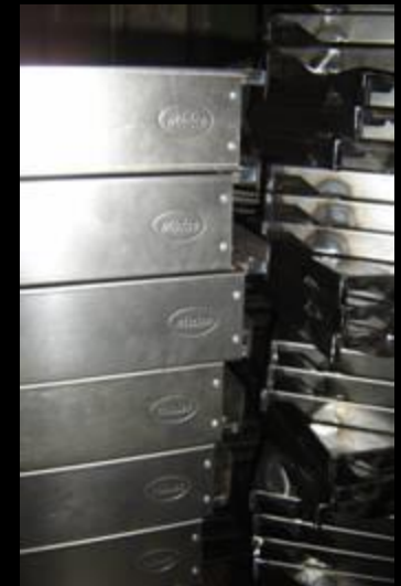
Emboss done during CNC punching
