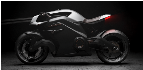
Fig 15. Arc Vector (2018) - Bold central volume, hub center steering, floating seat
