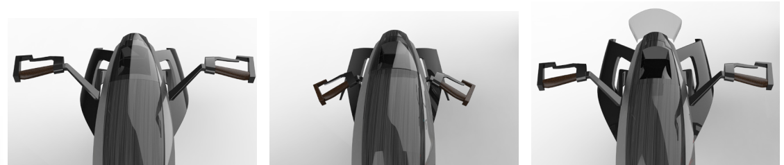
Fig 146. Different handle positions and transformation of upper fin in different modes - Urban, race, off-road
