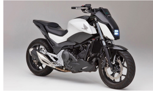
Fig 13. Honda Self-balancing motorcycle (2017)- Self balancing, self driving, AI assisted, conventional styling
