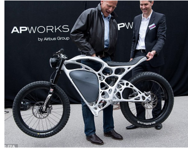
Fig 12. APWorks Light Rider (2016) - Generative design, 3D printed, extremely lightweight
