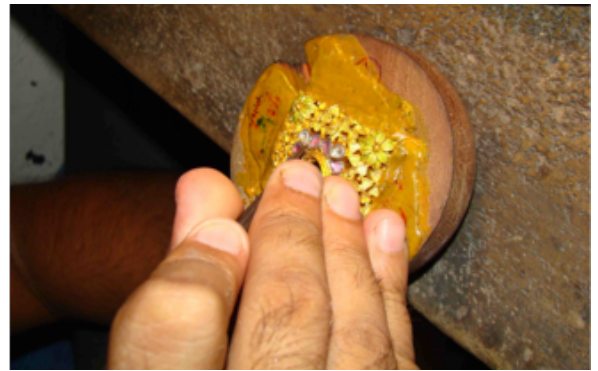
Fig.2.34. & Fig.2.35. A sharp tool is used for pressing that fuses gold by compression.
