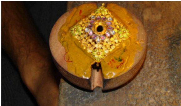
Fig.2.36. & Fig.2.37. Gemstones are set in place and excessive gold is trimmed off leaving a lustrous surface.
