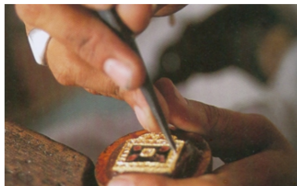
Fig.2.8 & Fig.2.9 An ornament ghat fixed on to a shellac stick to facilitate setting of gems.
