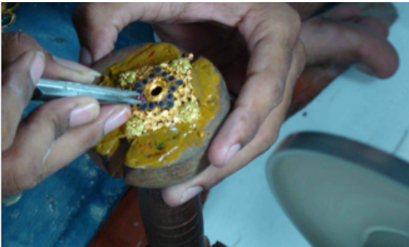
Fig.2.26. & Fig.2.27. Stones are finally fitted in their respective cavities and surma is applied to hold them.
