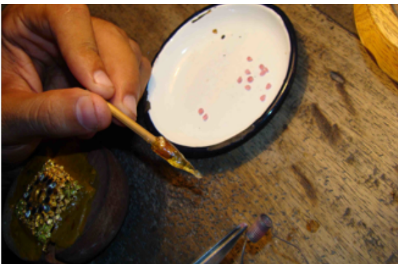
Fig.2.28. & Fig.2.29. Mild heat is applied to stones so it takes a proper seat in its bearing.
