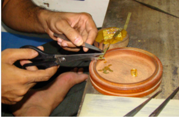
Fig.2.32. & Fig.2.33. A very thin foil is cut in small pieces and these pieces are pushed in cavities remaining between the stone and bearing.
