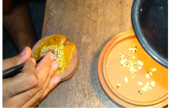
Fig.2.32. & Fig.2.33. A very thin foil is cut in small pieces and these pieces are pushed in cavities remaining between the stone and bearing.
