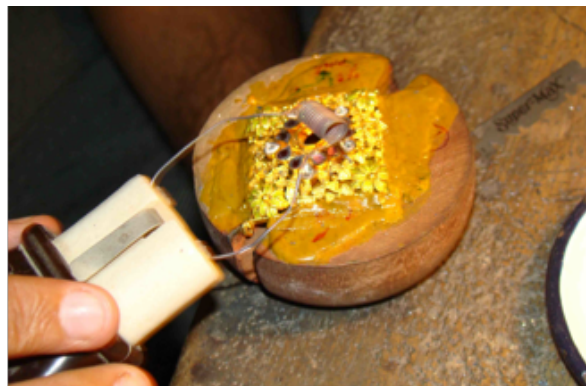
Fig.2.28. & Fig.2.29. Mild heat is applied to stones so it takes a proper seat in its bearing.
