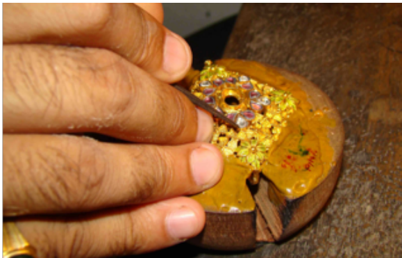
Fig.2.34. & Fig.2.35. A sharp tool is used for pressing that fuses gold by compression.
