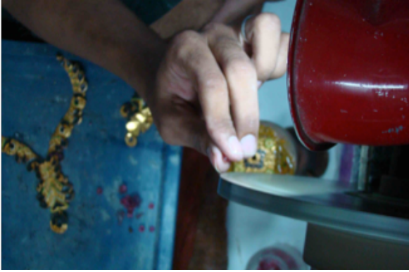
Fig.2.24. & Fig.2.25. Fine grinding of stones begets a good snug fit.
