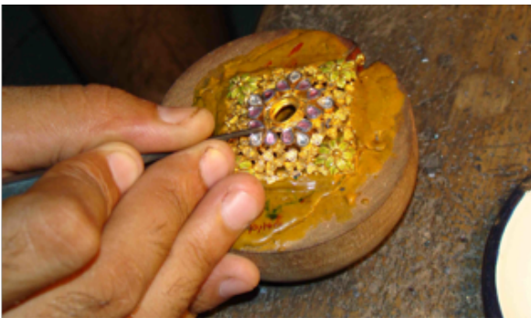
Fig.2.30. & Fig.2.31. Excess material is trimmed off & piece is ready for kundan setting.
