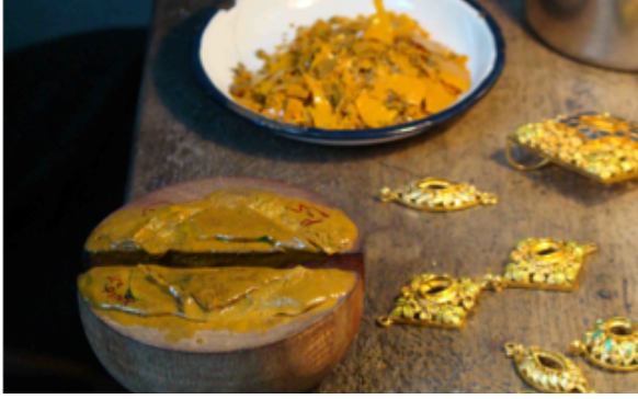
Fig.2.16. & Fig.2.17. Shellac flakes are heated and applied on a base.
