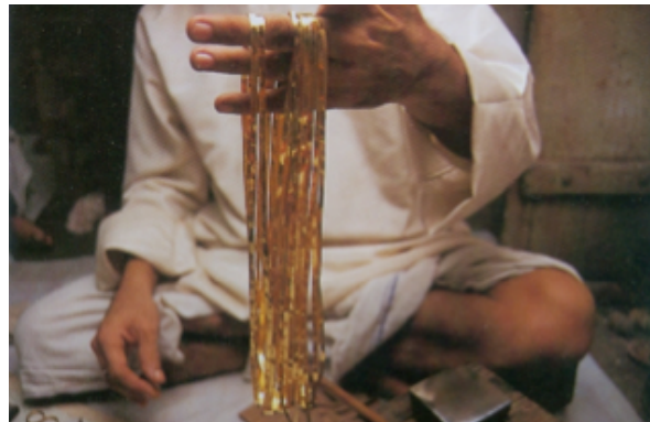
Fig.2.12. & Fig.2.13. Lengths of purified gold ribbon, ready to be used for kundan setting.
