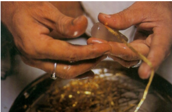
Fig.2.12. & Fig.2.13. Lengths of purified gold ribbon, ready to be used for kundan setting.
