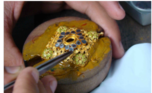
Fig.2.20. & Fig.2.21. Stones are placed in cavities to see fit and appearances, process is iterative.
