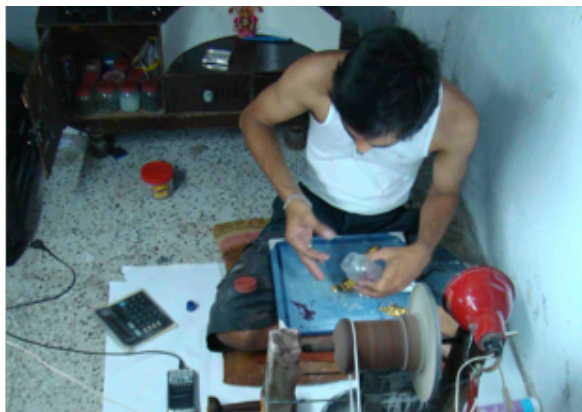
Fig.2.22. & Fig.2.23. Colored stones are custom polished for fitting.
