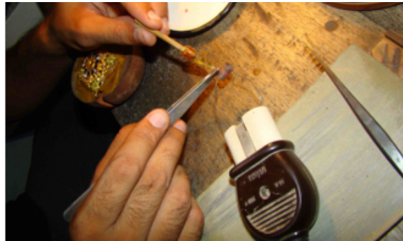
Fig.2.26. & Fig.2.27. Stones are finally fitted in their respective cavities and surma is applied to hold them.
