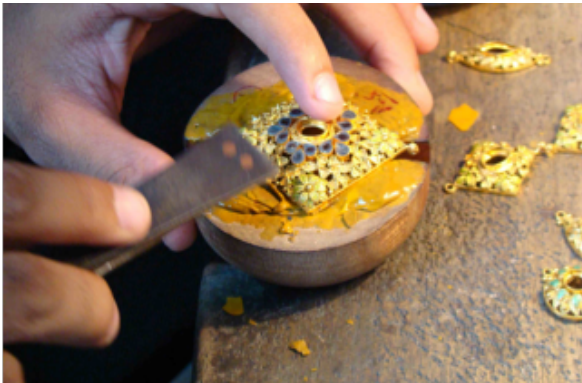
Fig.2.18. & Fig.2.19. An article is gently pressed in pliable shellac bed, heat applied for minor adjustments.
