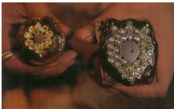
Fig.2.8 & Fig.2.9 An ornament ghat fixed on to a shellac stick to facilitate setting of gems.
