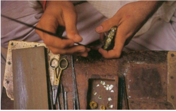
Fig.2.10. & Fig.2.11. The gem setter at work burnishing foils with an agate hammer.
