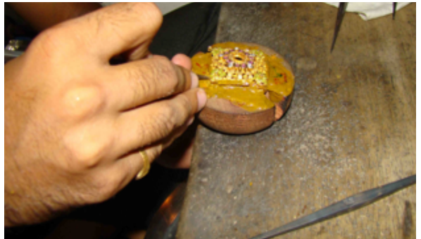
Fig.2.36. & Fig.2.37. Gemstones are set in place and excessive gold is trimmed off leaving a lustrous surface.
