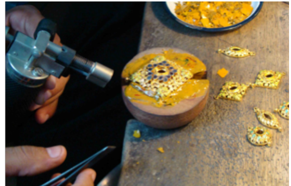
Fig.2.18. & Fig.2.19. An article is gently pressed in pliable shellac bed, heat applied for minor adjustments.
