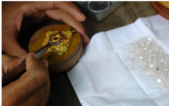
Fig.2.20. & Fig.2.21. Stones are placed in cavities to see fit and appearances, process is iterative.
