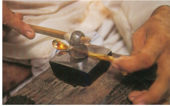
Fig.2.10. & Fig.2.11. The gem setter at work burnishing foils with an agate hammer.
