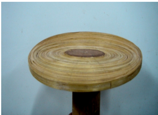
Fig. 11.13(b) Seat using coil technique
