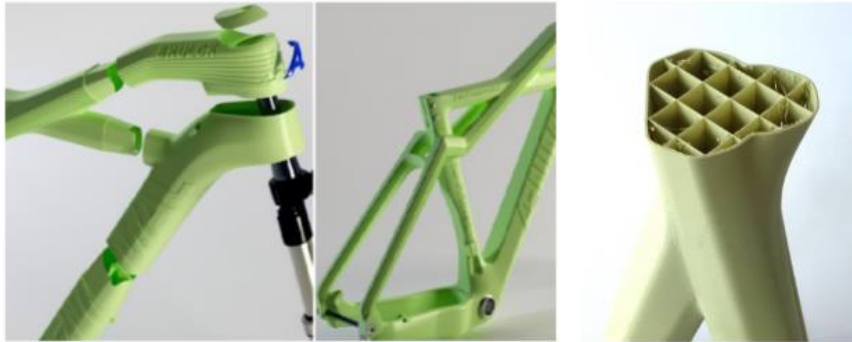
Bhulk 3D Printed, Compostable Bike Frame
