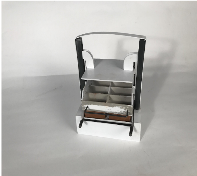
Fig 101 : cover plate is provided above the mould which also slides in the same channel
