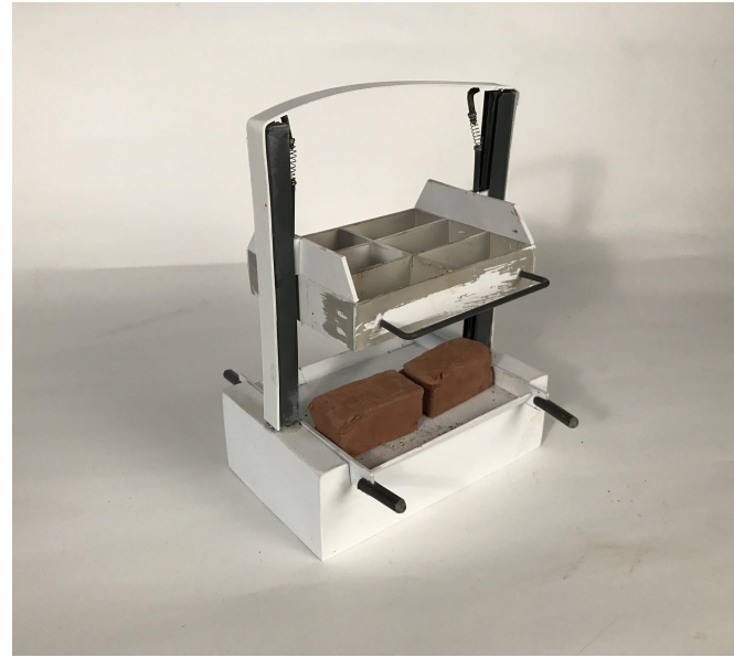
Fig 100 :vertical sliding tray which is spring loaded
