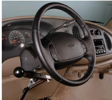
Figure 11 Car modified with all handle control
