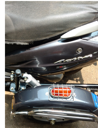
Figure 17 Indication bulb on side wheels
