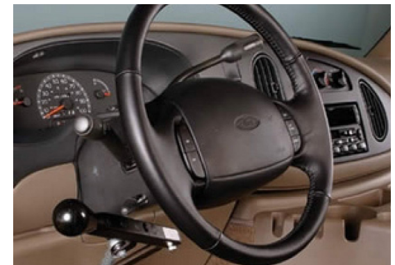
Figure 8 Car modified with all handle control
