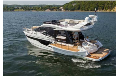
Img 30. Folding out balcony
