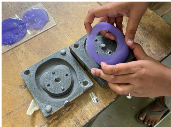
Fig 52. Demolding the cast
