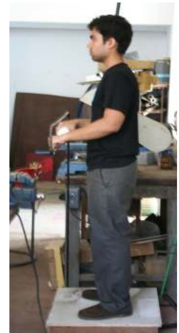
Mock up rig showing the minimum area required for a single person to stand
