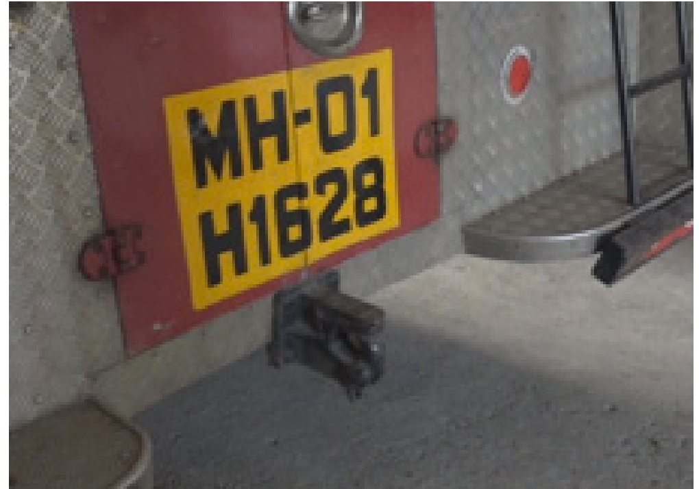
Towing hook incase another vehicle is stalled
