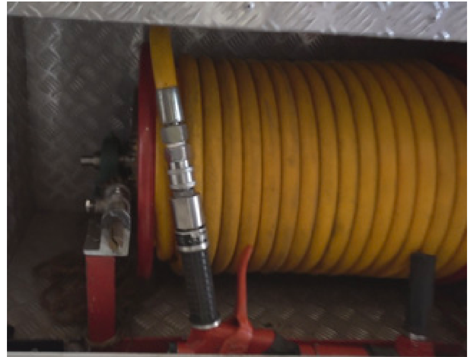
mini fire hydrant which is directly connected to the water tank through the pump. This one has a gun type nozzle.
