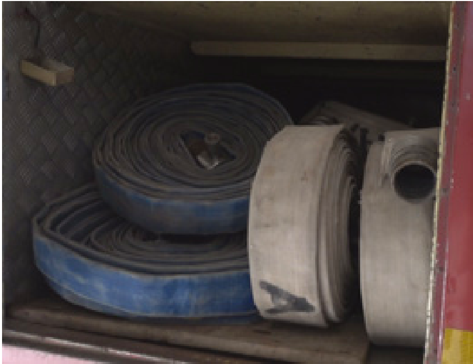
White hose: main hose with universal clamp
