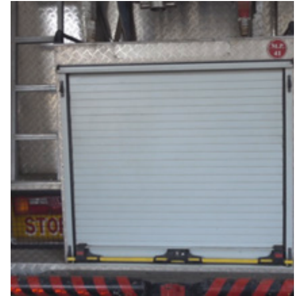
quick release shutter to access the main pump
