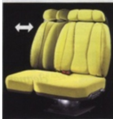
Extending seat backs (satellite seats)
