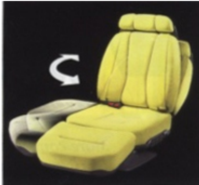
Front rotating satellite seat
