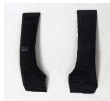
Image 34: 3d printed L.E.D housing to check the optimum vein viewing area
