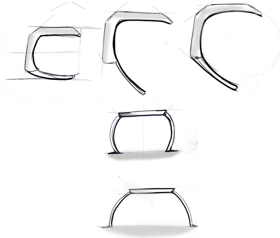
Image 37: Clamping mechanism and its range of expansion Source: Author
