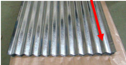
Figure 5.1: Galvanised roof sheets
