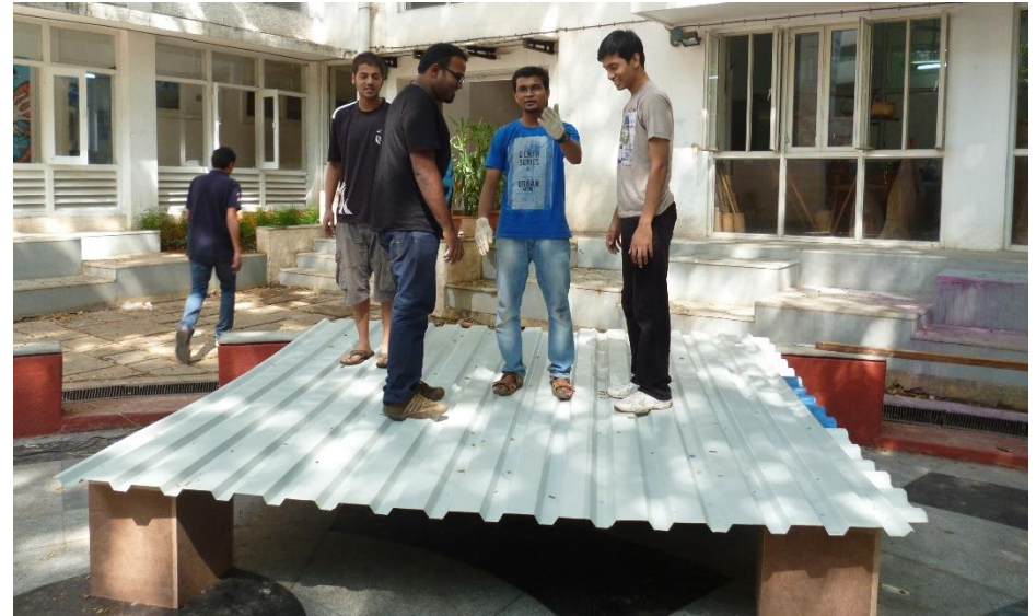
Figure 8.8 Strength testing for bending
