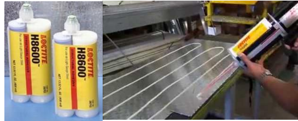
Figure 7.13 Adhesive for sheet metal joining
