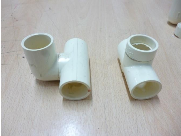
Image: redesigned 'Tee' (left) existing 'Tee' (Right)
