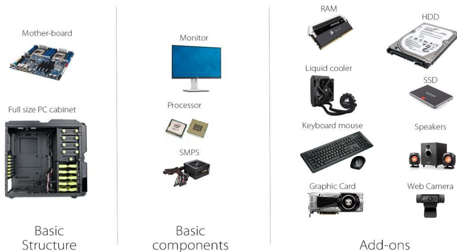
Figure 18: Personal computer components
