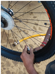
Spoke wrench being used to adjust the spokes
