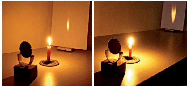
Image formed by Concave Mirror
