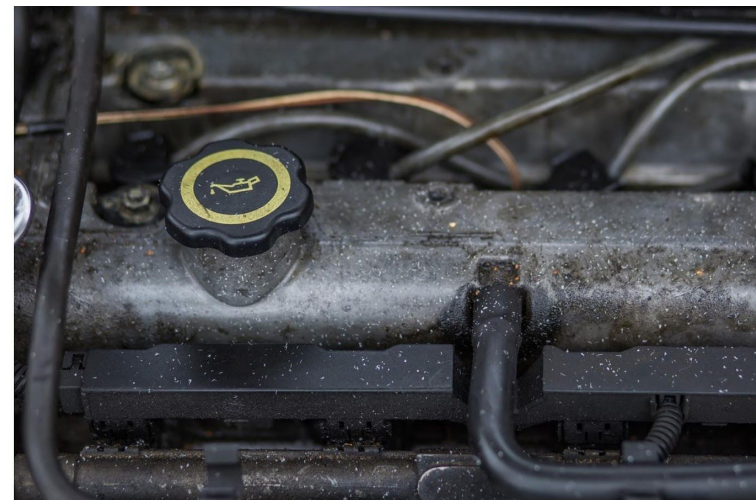
Fig 2: Cap of the engine oil tank to which the measuring stick is attached
