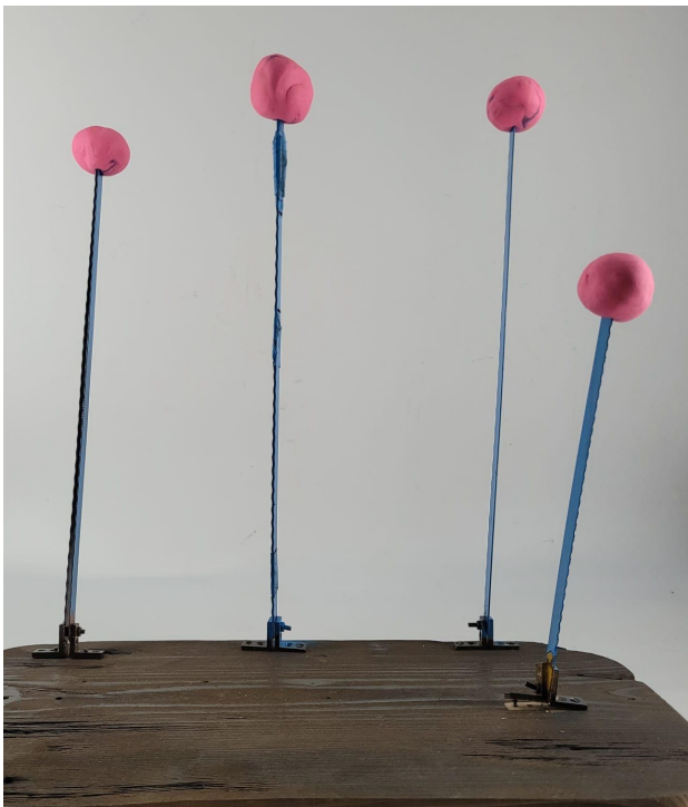
Masses on top of structure to reduce the damping of the
