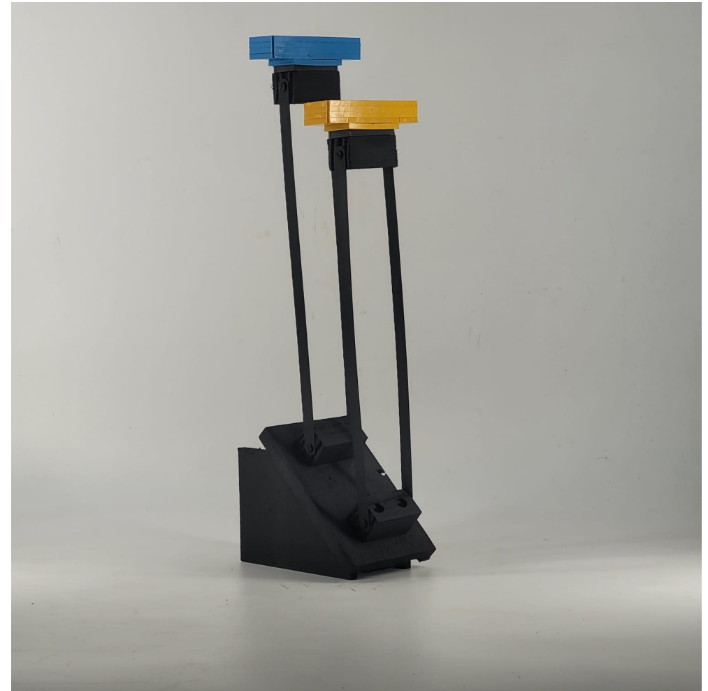
The incline position of the base replicates the hand and mass damping is only possible when the masses are normal to the ground
