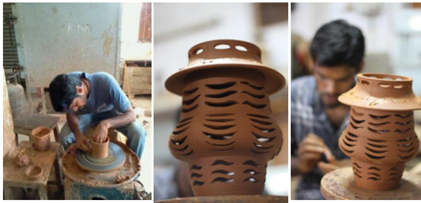
Fig.15.2 basic shape of the product is achieved by throwing process. Product is done by three parts by throwing and assembled them together by using clay slip.
