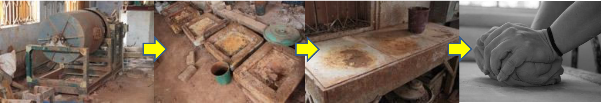
Fig 15.1 1) Mixing and grinding the clay in Ball Mill 2)Drying on plaster of paris block 3) Wedging: Wedging is the process of mixing the clay by hand by rotating and pressing a clay ball on a table. The purpose is to thoroughly homogenize the clay and to remove all air bubbles. This is particularly important, as the presence of air bubbles in the clay will result in explosions in the kiln as the air pockets expand and burst
