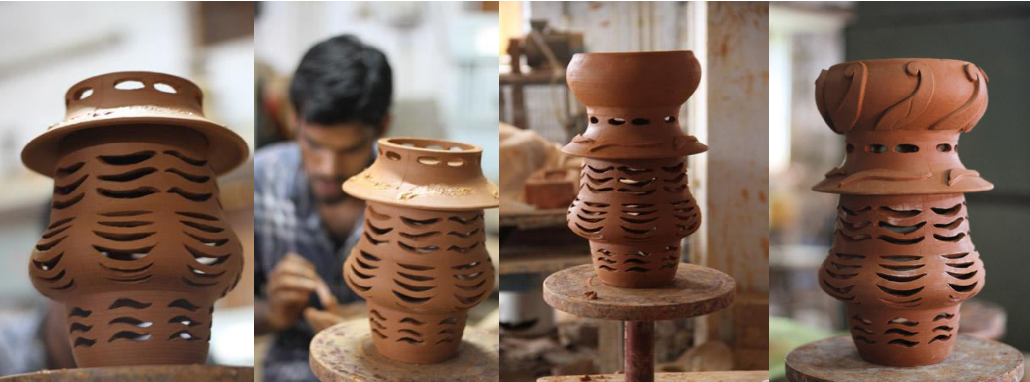
Fig.17.1 Decorating and piercing the product using slab making process and knife
