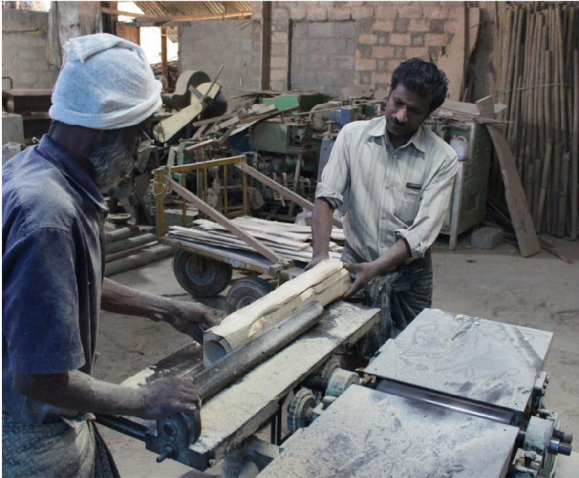
The machine room at uravu where the resources are cut down to various sizes according to the need.
