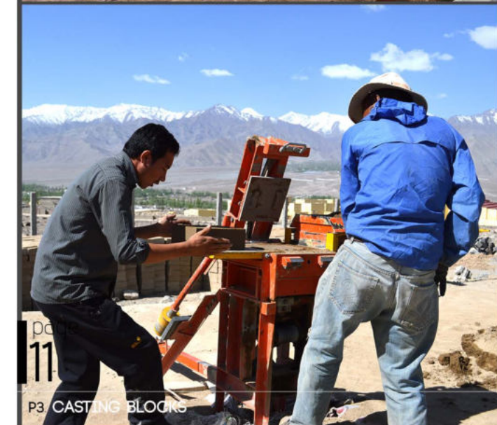
P2. AURAM 3000 CSEB CASTING MACHINE AT RBC
