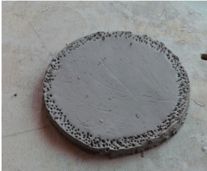
Pricking of slab and applying slip for attachment
