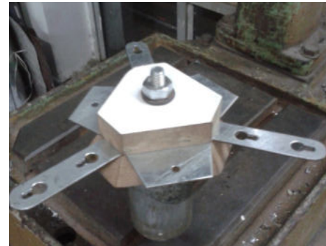
tightening the metal sheet between the fixture
