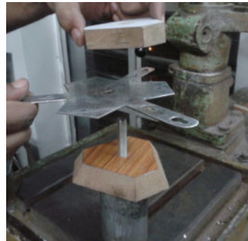
Fixture to bend it at 60 degree angle
