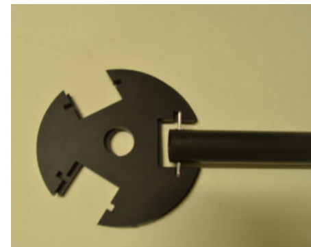
By using small acrylic fitting as shown in the figure tetrahedron vertices can be joined together.
