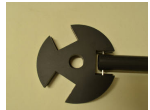
By using small acrylic fitting as shown in the figure tetrahedron vertices can be joined together.
