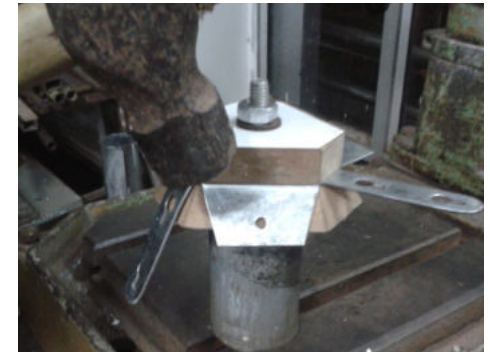
bending it at the required angle with the help of a hammer.
