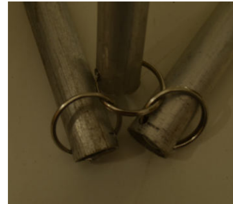
In order to figure out fastest n cheapest joinery to join tetrahedron vertices together, it can be interlocked by small metal rings.
