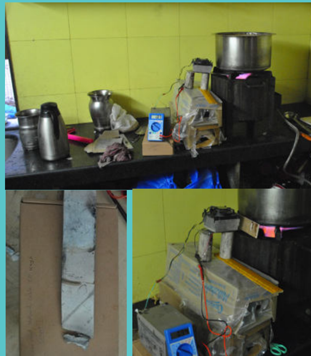
Experiment with commercial gas stove and fan cooled sink.
