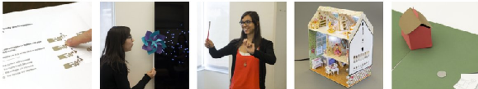
Figure 1. Left to right: A wireless polling device, a pinwheel animation that adapts with spin speed, a conducting baton, a dollhouse controlled with custom RFID tags on paper interfaces, and a pop-up book with embedded tags which trigger audio content.
