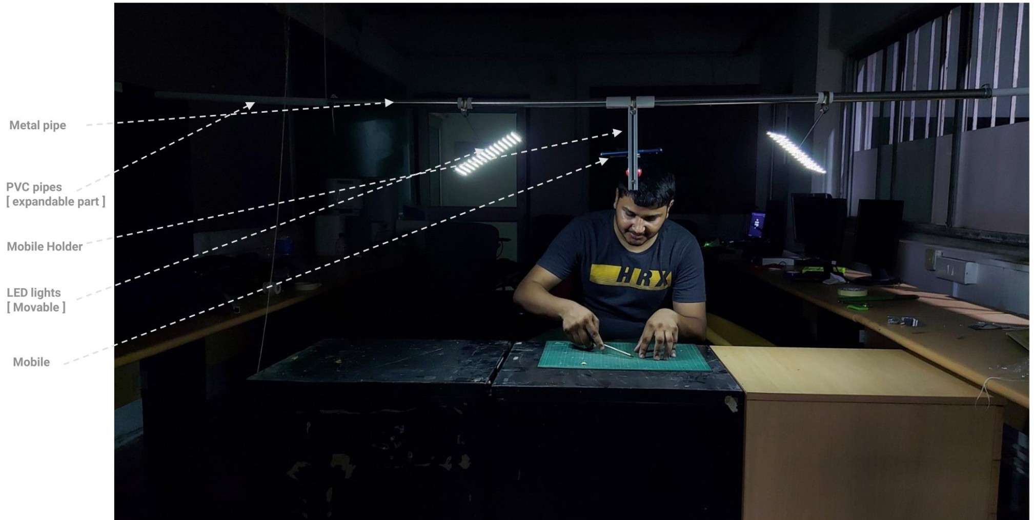
Fig 148 . Mock up testing
