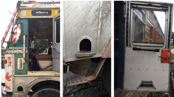
Fig 24. Ingress and egress in the truck. A small improvisation made build by the drivers.
