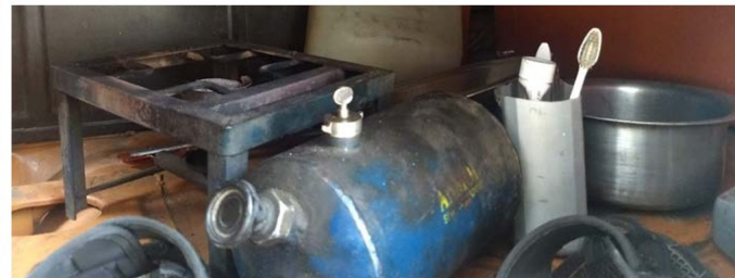
Fig 40. Picture showing kerosene stove under co-driver seat.
