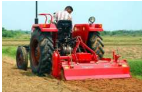
Rotavator to pulverise the soil
