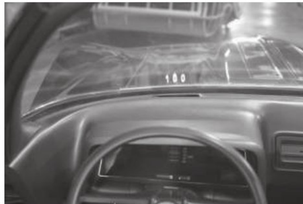
Fig.2: (Left) An early head-up display in a Chevrolet Corvette XP-856 Aero Coupe concept car from 1965 or 1966
