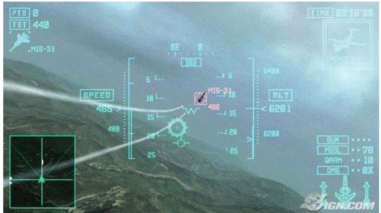
Fig.5: HUD in modern day fighter jet aircraft. It is a combination of static and volumetric projection of data. The target lock symbol will always stay in the line of sight between the pilot and target by using head tracking.
