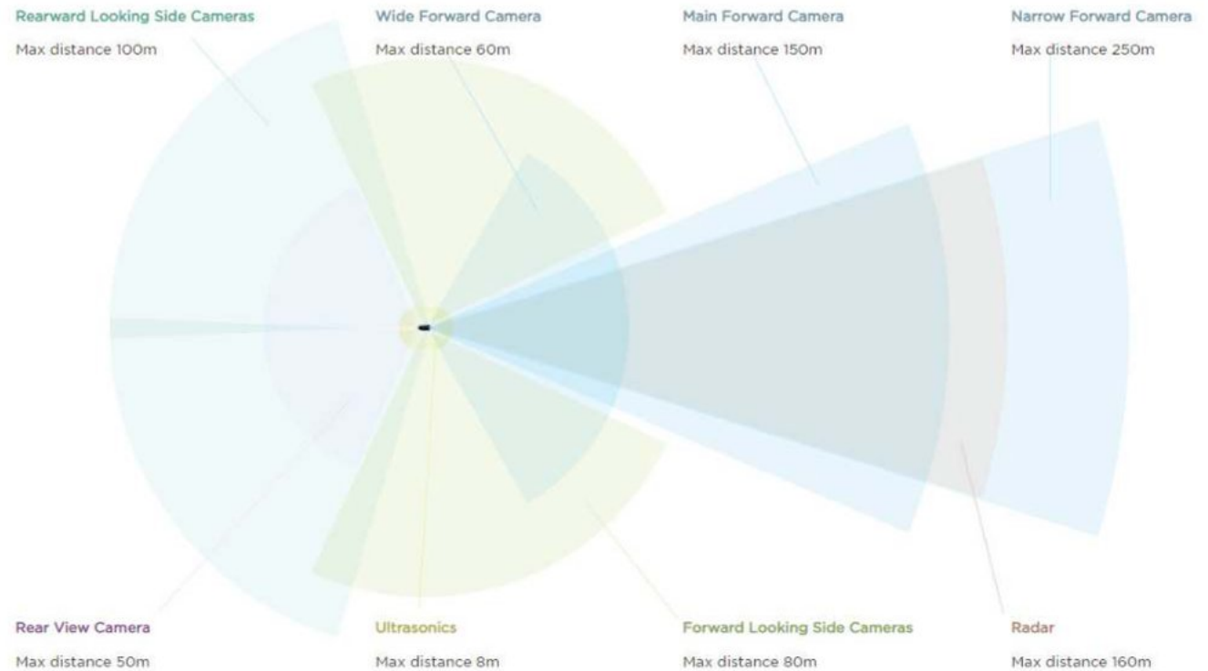
Fig.14: Tesla's vehicle's currently uses several sources of data to acquire autonomous driving: radar, GPS, maps, ultrasonic sensors and more. But not lidar like some of Tesla's chief competitors.
