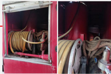
DCP set up with it's own pump and the hoses
