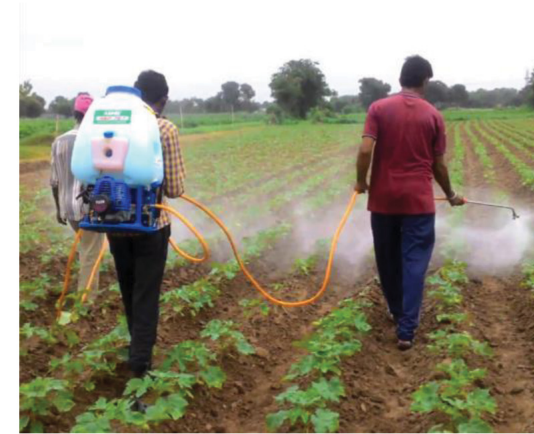
Fig 1.13 Knapsack power Sprayers, Capacity: 20 liters
