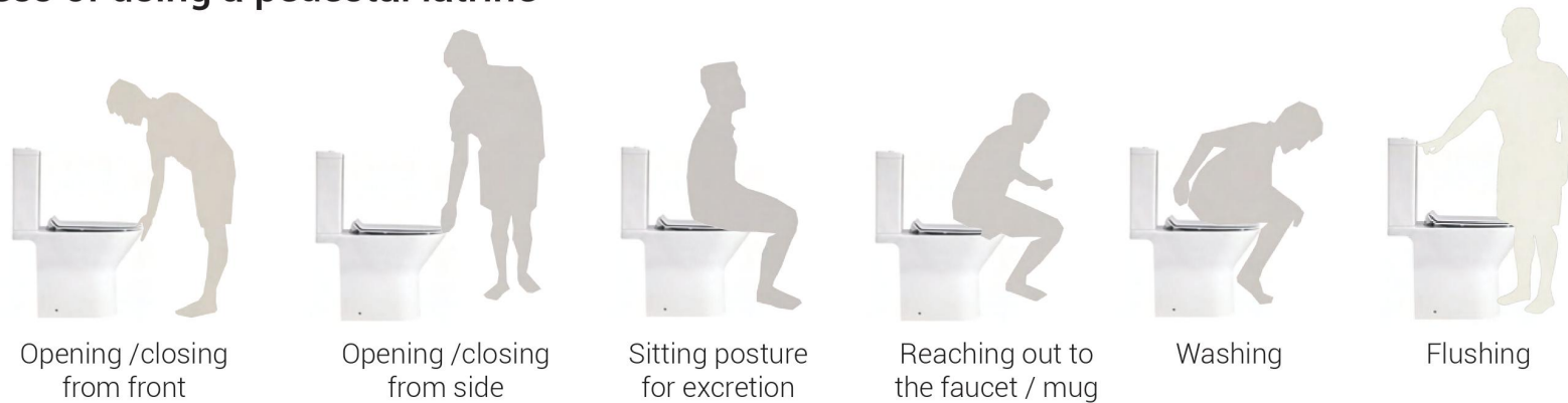
Fig.49. Operations performed while using pedestal latrines
